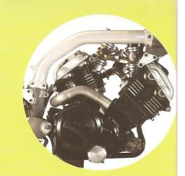
With an engine capacity of 996 cc and a chamber angle of 72°, the engine architecture is used on all models to ensure unbeatable power, drive and character.
